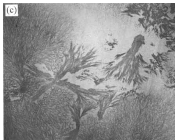
Figure 8 TEM images of fully cured polymer blend films ( \times 10^4 ) (a) 30/70, (b) 50/50, and (c) 70/30 (COPNA/nylon 6).
